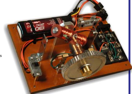
Now the side that was positive becomes negative, and the negative becomes positive. This makes the electromagnet change the poles, N to S and S to N. Now the electromagnet poles are the same as the permanent magnets and they want to move away. See the right figure. This keeps the rotor turning until the electromagnet reaches the other side and the commutator changes the electricity again. This keeps repeating and the motor keeps running as long as the battery is connected.
